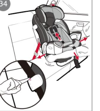
**33 Safety Check for Secure Installation**
